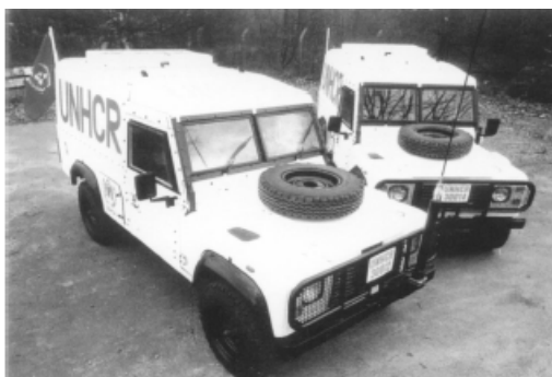
Figure 5.22 Armoured Land Rovers (CAV-100) with body armour based on S-2 glass fibre panels produced by National Plastics
