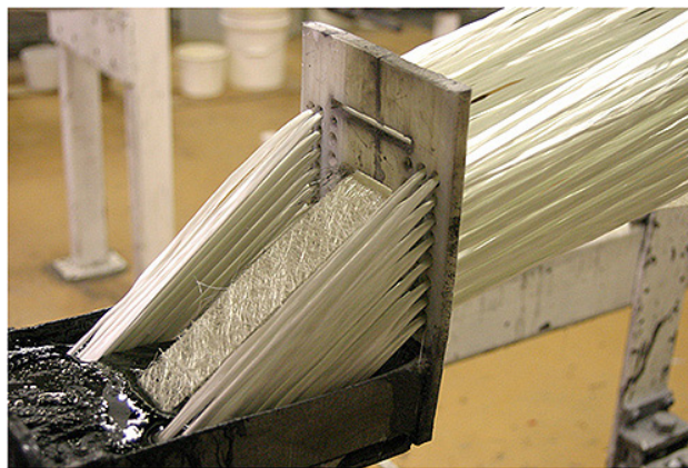
Figure 2.14 Open-bath pultrusion forming (source: Martin Pultrusion)
